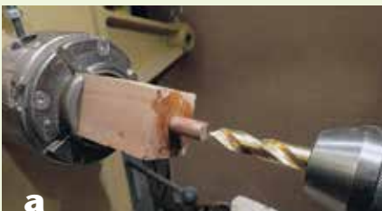
a Drill wood blank and glue in dowel.
