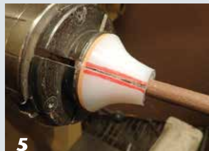
5 In use, be sure this gap (marked in red) is aligned with one of the gaps between the metal jaws of your four-jaw chuck; this allows the collet chuck to close properly.
