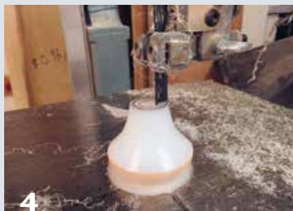
4 At the bandsaw, cut a 1/8"-wide gap in one side of the collet chuck.
