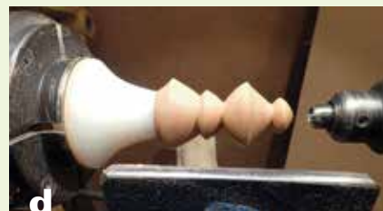
c Turn your bottle stopper shape. No worries if you cut into the plastic collet chuck. Keep the tailstock in place for support until your final cuts on the end.
