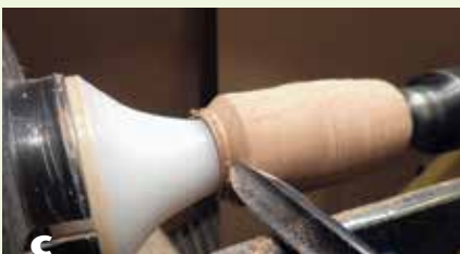
c Turn your bottle stopper shape. No worries if you cut into the plastic collet chuck. Keep the tailstock in place for support until your final cuts on the end.
