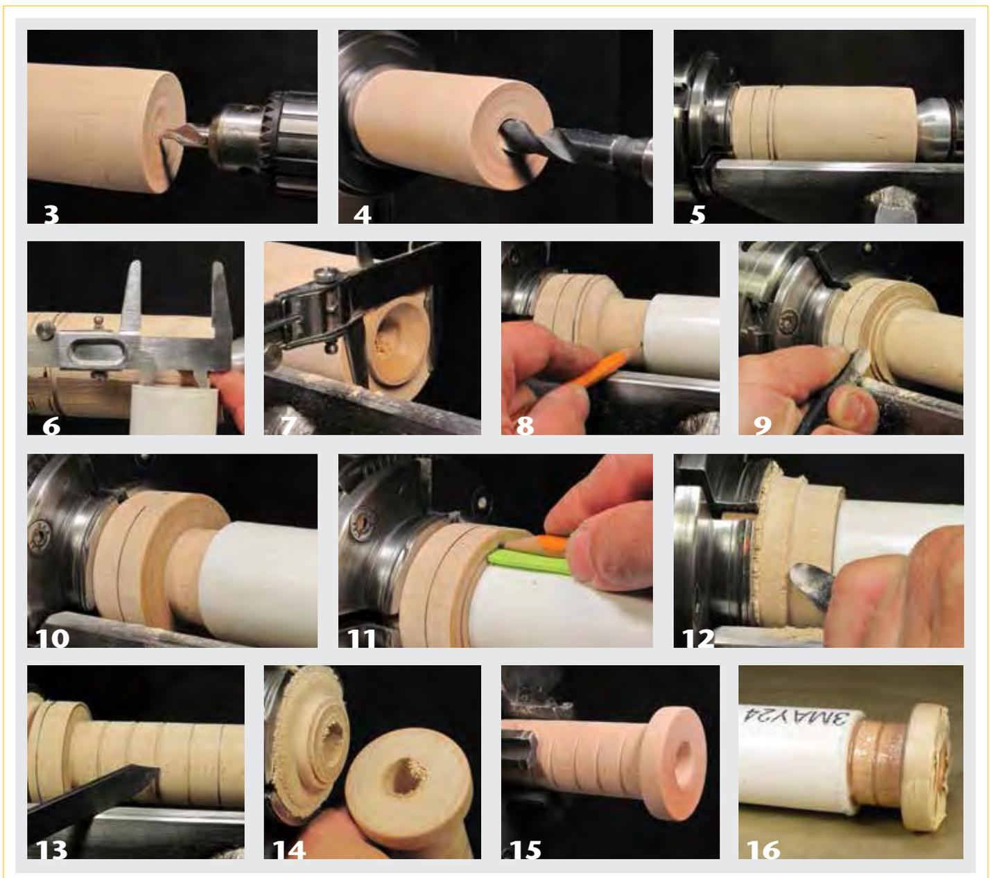
of your blank (*Photo 7*). Test fit this section to your PVC pipe before roughing out the rest of the tenon with a spindle roughing gouge.
