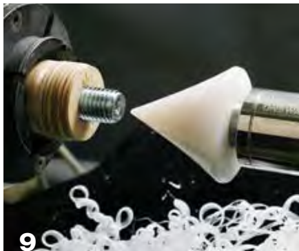
9 The custom cone, mounted on a Oneway live center, is ready for your next project.
