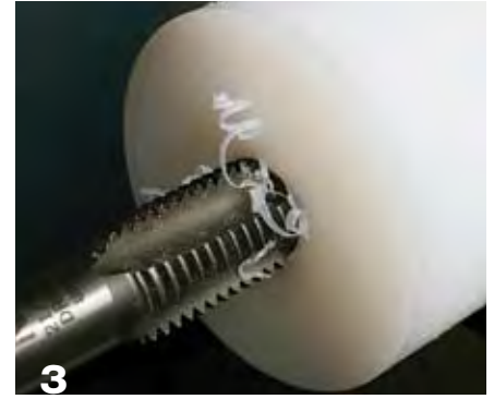
3 Tap ¾"×10 thread. For more details, see "Hand-Threading on the Lathe" opposite .
