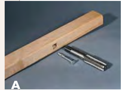
A Make a homemade tap handle from 1\frac{1}{4} x 1\frac{3}{4} x12" hardwood with a \frac{7}{16} "-square hole and \frac{1}{4} x 1\frac{3}{4} " bolt.
