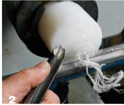
2 True up the UHMW blank with a bowl gouge and create a recess to start the drill.
