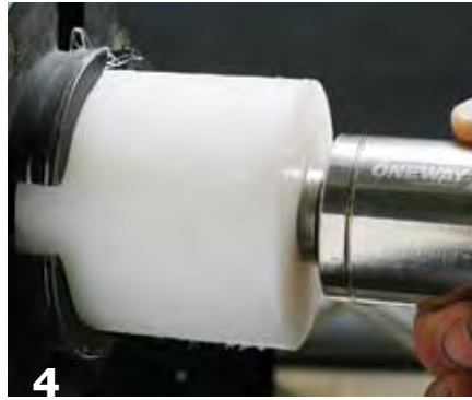
4 Test the new threads. The blank should seat square and tight against the live center.
